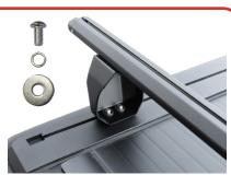
Load bars onto the truck bed for the final step. Insert 4 nuts into each rail. Lock all 4 boxs to the nuts on the rail with one screw, ring, and washer using L-wrench. Done!
