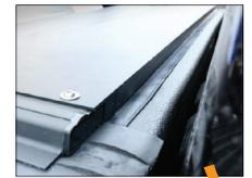
3b. With two people, lift the cover assembly and place it onto the truck bed, starting by placing the canister portion near the bulkhead. The front seal of the cover should be laid flat, not tucked in.
